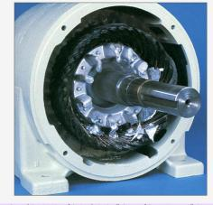
Severe thermal deterioration of the insulation in all phases of the motor normally is caused by very high currents in the stator winding due to a locked rotor condition. It may also occur as a result of excessive starts or reversals.
